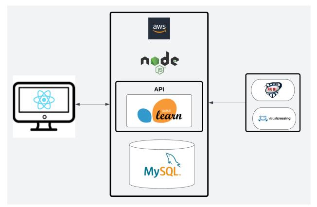
When a user first tries to enter the site, a DNS lookup is performed, after which a simple GET request is made to the HTTP server that serves the React application. The application is sent to the client's browser, after which point it is used to request data from the server. When a
